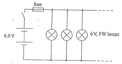
The fuse is rated at 13 A. This means the fuse will "blow" if the total current through the circuit exceeds 13 A. When the switch is closed in the above circuit, determine the maximum number of 6V,9W light bulbs that can be added in parallel without the fuse blowing.
